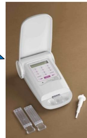
Determine step protein concentration yield real time on the floor without sample dilution
